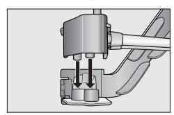
■ Now push the milk pipes into the guides (①) and push the spout holder (②) back on. It should click into place.
